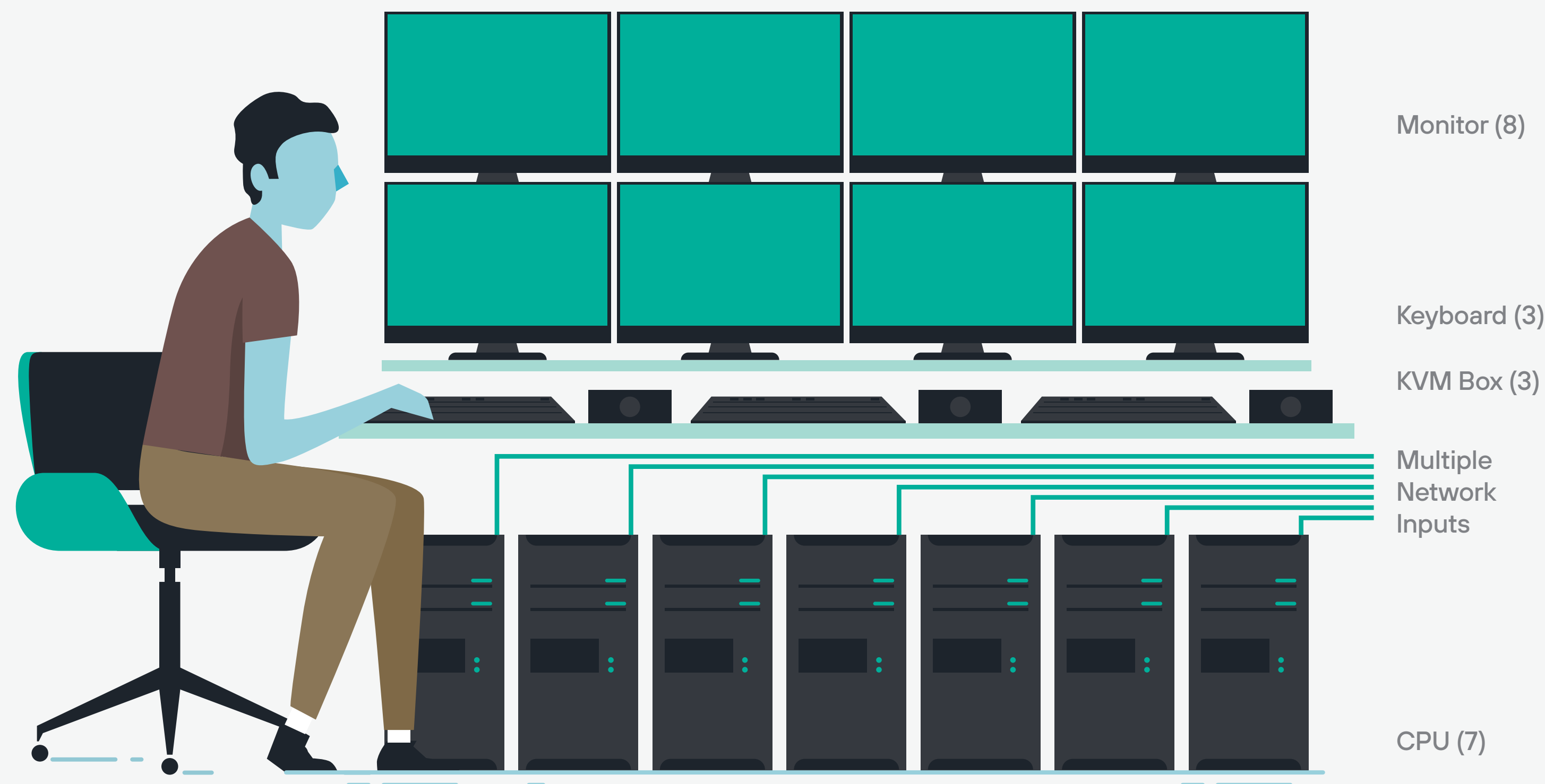
Figure 2 - Typical Workstation Setup for Multi-Domain Operations in Classified Environment
